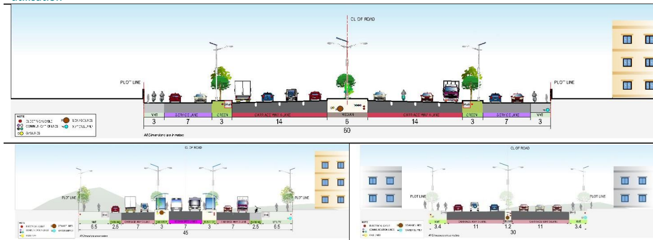
Figure 14-34: Hierarchical road network of RoWs of 60m, 45m, 30m, and 24m will be planned in VMR to streamline the mobility and safety aspects.
