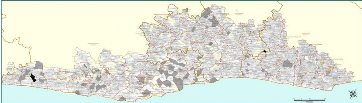
Figure 6-5: Geo rectified revenue village map superimposed on ortho-rectified satellite imagery
